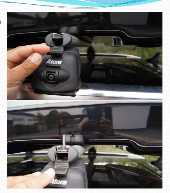
Lift the box and place the T-adapter in each case under the slot
